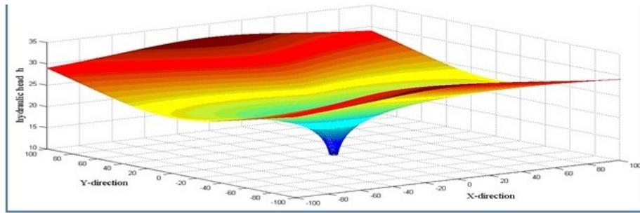
(a) The hydraulic head with  $T_x = 150, T_y = 90$ .
