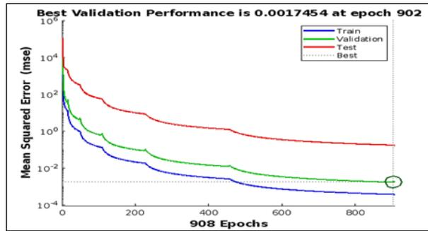
Figure 4: Comparison between training, testing and validation results for ANN.
