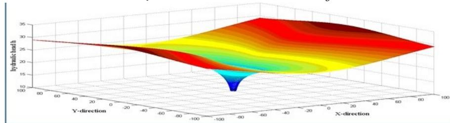
(b) The hydraulic head with  $T_x = 90, T_y = 150$ .
