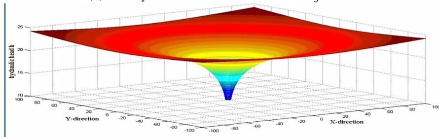
(c) The hydraulic head with  $T_x = 150, T_y = 150$ .
