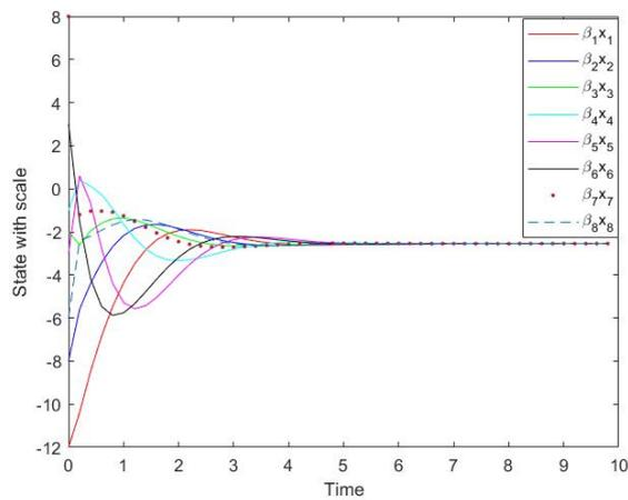
Figure 3: The state trajectories scalar scales  $(2, -2, 1, -1, 3, 1.5, -2, -1)$  with  $h = 0.2$ .
