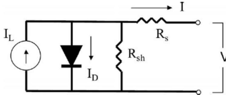
Figure 2. Equivalent electrical circuit in the five-parameter photovoltaic model [14]
