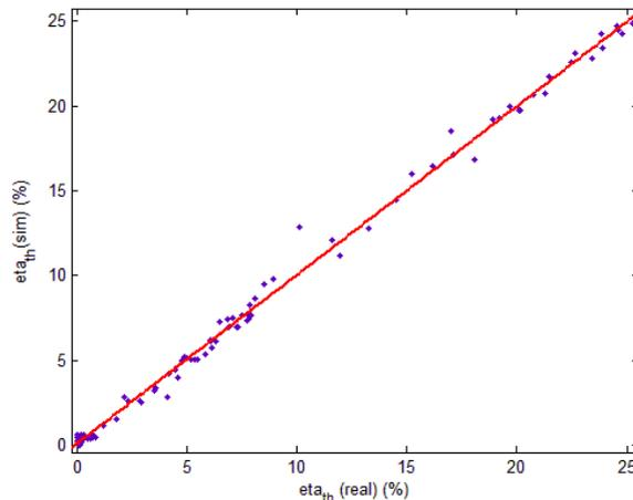
Figure 4. ANN simulated thermal efficiency vs. experimental value
