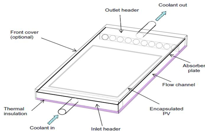
**Figure 1. Main features of a flat-plate PVT collector [3].**
