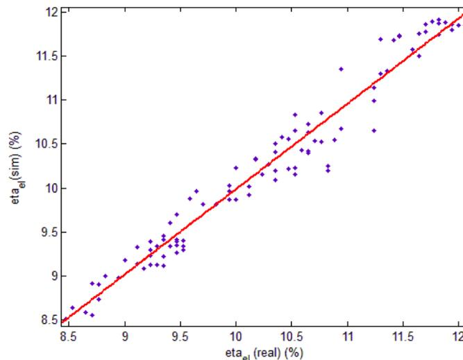
Figure 5. ANN simulated electrical efficiency vs. experimental value
