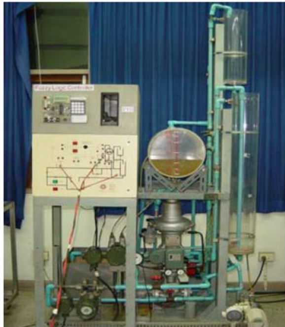
Figure 1. Plant level control set up [5]
