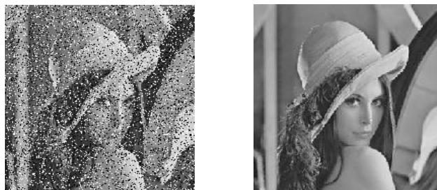
Figure12: noisy image with intensity of 0.2 and the result of applying optimized fuzzy filter.
